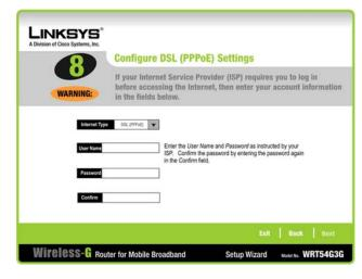
Figure 7-11: Configure DSL (PPPoE) Settings Screen
